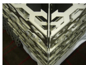
Pictures left/centre: Corner pieces with mitre cuts and toothed blades as protection
